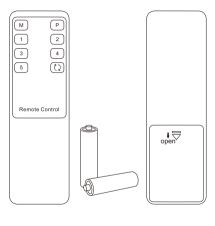
**Tips:** By default, the remote control is not equipped with batteries, due to the safety requirements of some express companies. Install AAA dry cells before use.
